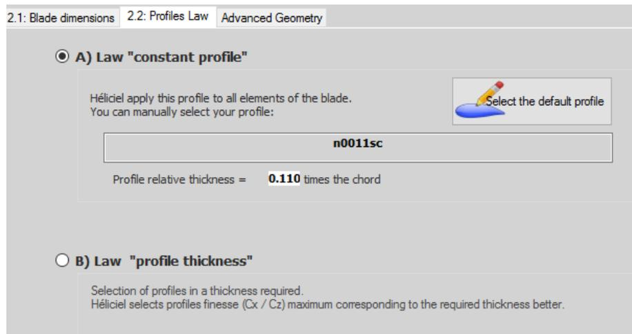
In constant profile default profile is selected by clicking the tab on the right side. Heliciel has Interactive profiles database from which one can select with a larger variation in Renoyld's No. i.e., 10000 to 5000000.
