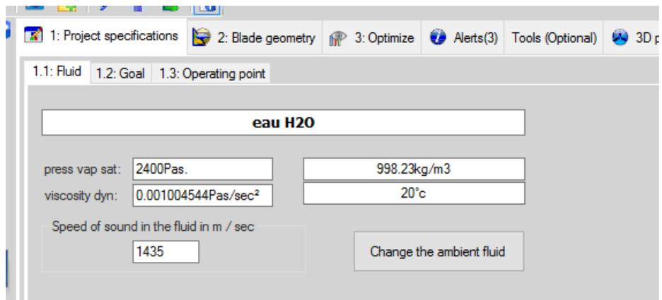
By clicking on the change the ambient fluid tab, a new window appears where we can select the type of fluid and ambient temperature of the fluid as shown in below figure that water has been selected with temperature of 20 °C.
