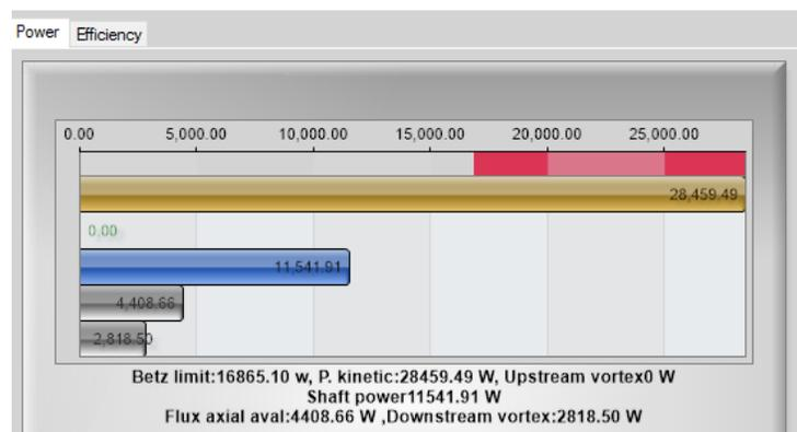
Efficiency is the ratio of shaft power to kinetic which is available power and it is 0.406.
