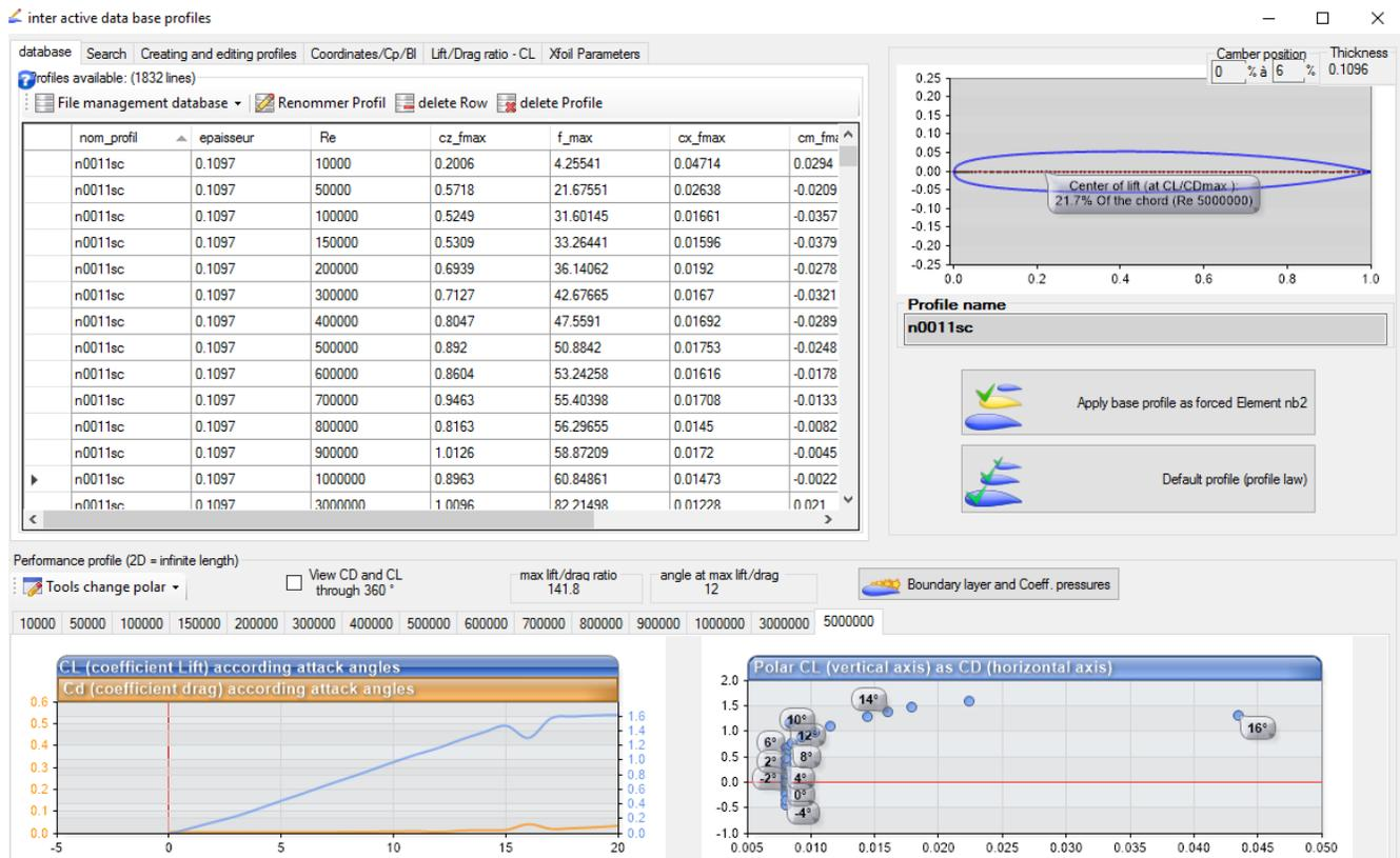
Also there are two options here whether we want to examine default profile for each element of blade or for specific element of the blade for example in the above figure it is shown that there is an option to select the profile for just blade element no. 2, not for the other elements of blade.
